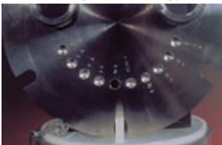
Picture 3: Locating holes with locating pin
